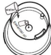
**⚠ Pls do not exceed the maximum water level, two or three drops of essential oil is enough for 110ml tank**
