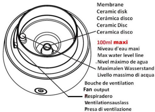
Clean the ceramic disk and the water tank with soft cloth or cotton sticker in clean water with some white vinegar. Also, you can place 2 to 5 drops of white vinegar on the ceramic disk and leave for from 2 to 5 minutes.
